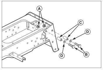
Figure 3. Install Rear Spacers
